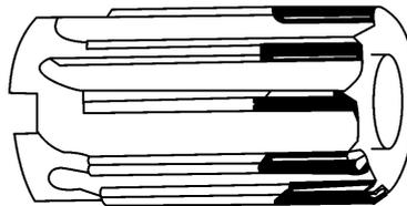
*Fig. 3.15, A carbide tipped shell reamer.*
