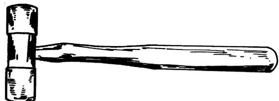
Fig. 2.21 (b), Plastic faced soft hammer.
