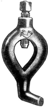
Fig. 6.23, Bent-tail lathe dog.
