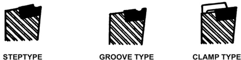
Fig. 4.8, Chip breakers
