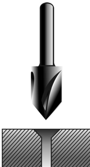
Fig. 3.26, Countersink and countersunk hole.
