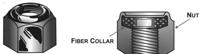
*Fig. 15.9, Low-temperature (250°F or less) self-locking nut (elastic stop nut, AN 365, MS20365)*
