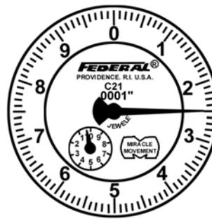
Fig. 2.69, Continuous dial with revolution counter and double dial.
