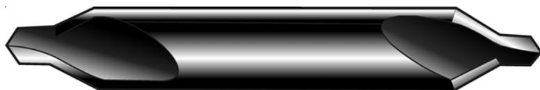
Fig. 3.27, Combined drill and countersink.
