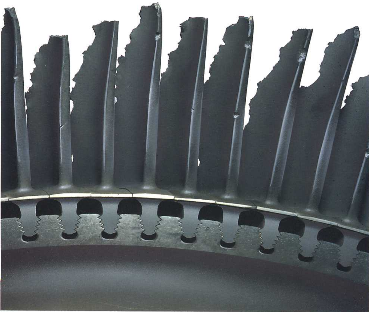
Fig. 24-9 Overheated turbine blades.
