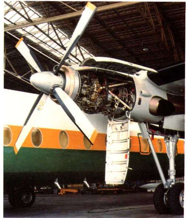
Fig. 23-13 Engine accessibility, turbo-propeller engine.
