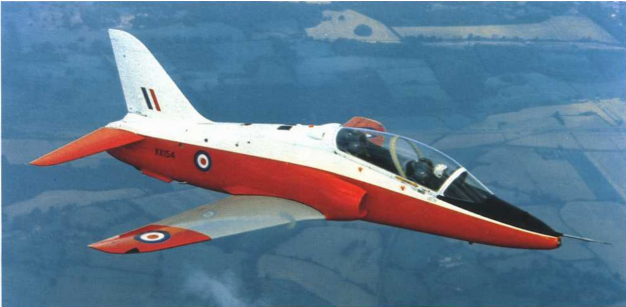
Fig. 23-6 Single engined aircraft with fuselage intakes.
