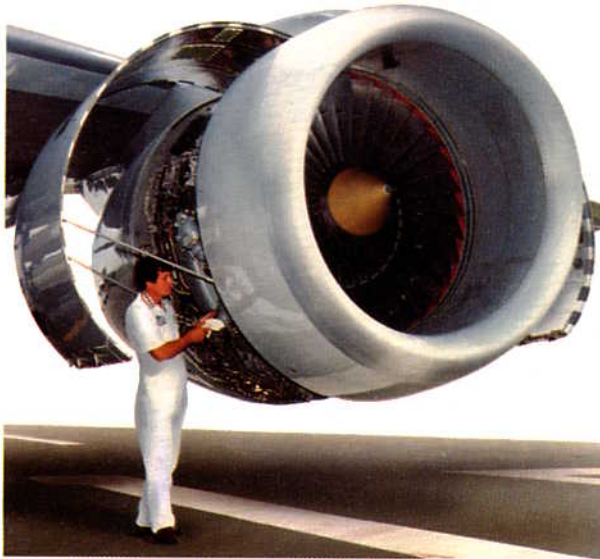
Fig. 23-12 Engine accessibility, turbo-fan engine.
