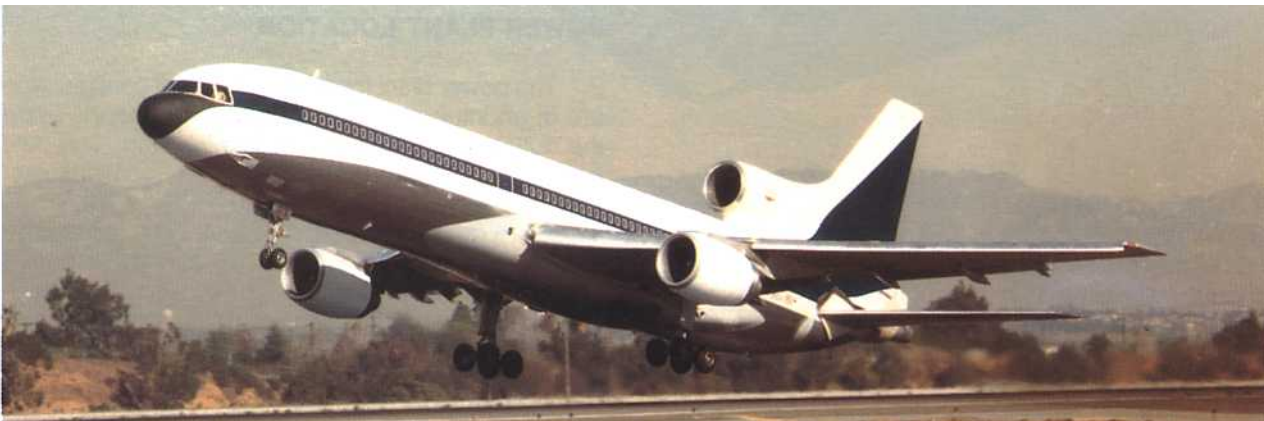
Fig. 23-3 Tail and wing-mounted pod installation.
