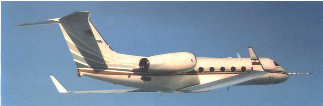
Fig. 23-2 Fuselage - mounted pod installation.
