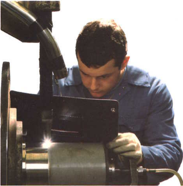
Fig. 22-8 Tungsten inert gas welding.
