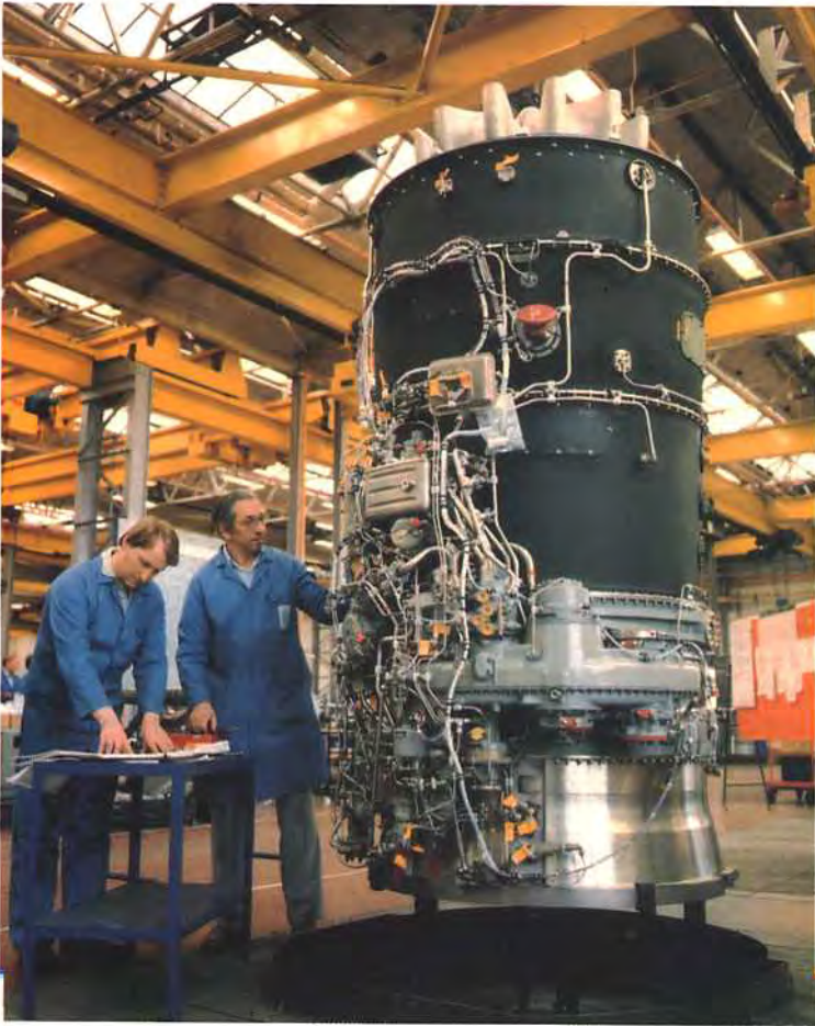
Fig. 25-10 Engine assembly --- vertical.
