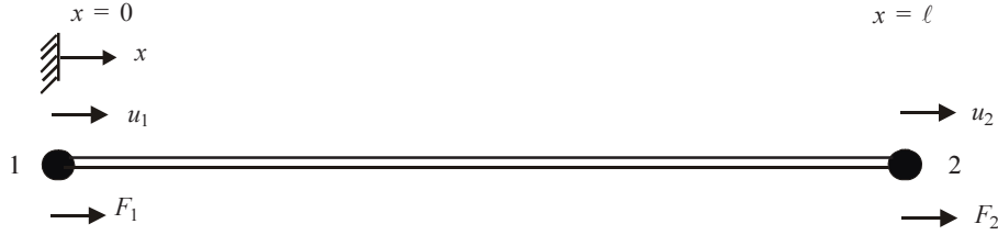
Fig. 3.7 Typical bar element.
