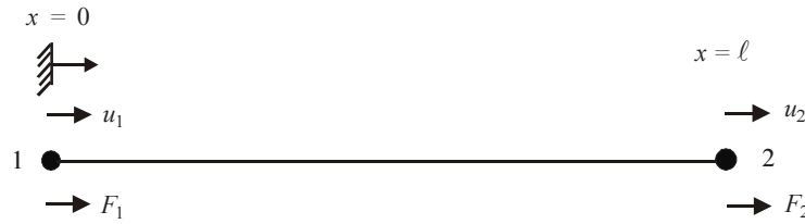
Fig. 6.4 Typical bar element.
