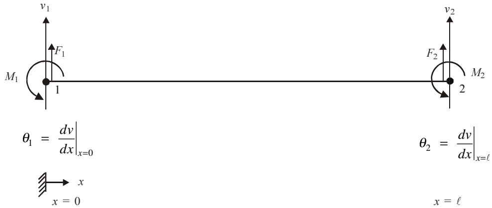
Fig. 3.9 Typical beam element.
