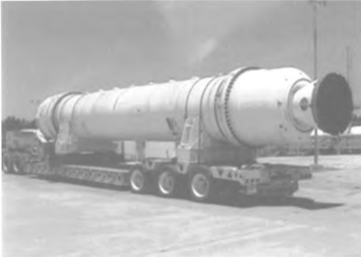
FIGURE 15-3. Static tests of a 250,000 lbf thrust hybrid motor prototype demonstrated that additional work is needed to understand fuel regression and combustion stability issues at large scale. The fuel case shown here is approximately 6.3 ft diameter.
