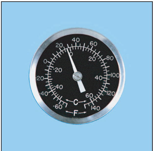
Figure 6-24. Outside air temperature gauge.
