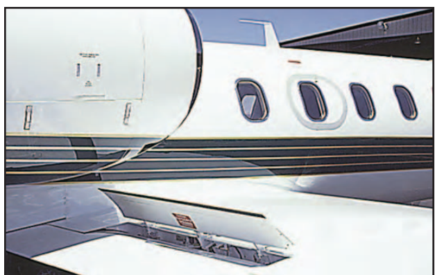
Figure 4-15. Spoilers reduce lift and increase drag during descent and landing.
