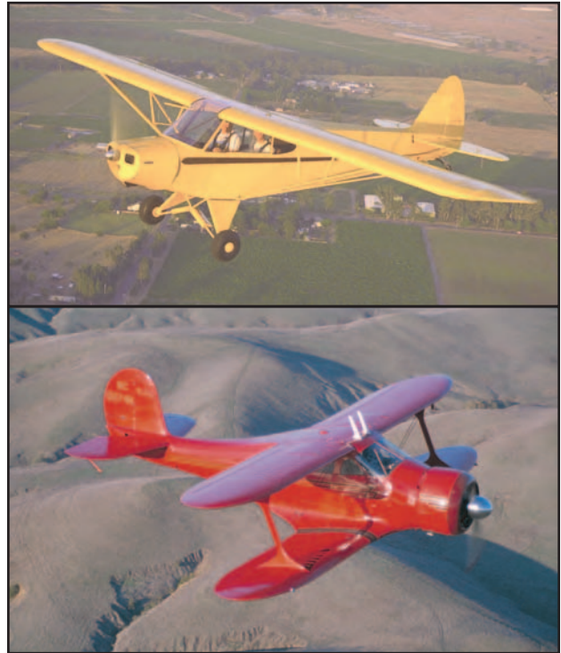
Figure 1-5. Monoplane and biplane.
