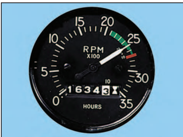
Figure 5-5. Engine r.p.m. is indicated on the tachometer.
