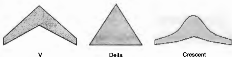
Fig. 11.18 Swept-back wings for transonic speeds
