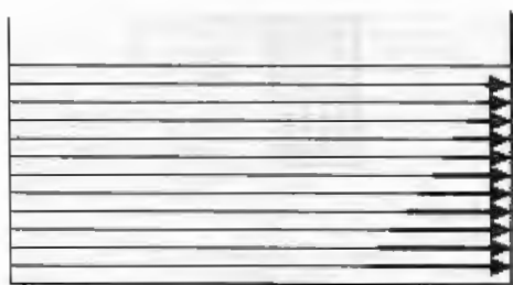
Fig. 1.9 Pressure increases with depth below the surface
