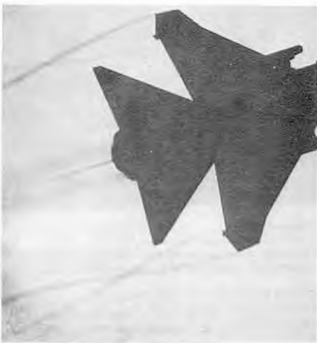
Fig. 3B Rolling up of vortices on TSR2
