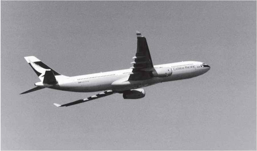
Fig 9C Sweepback An Airbus A330 showing the sweepback of the wings.
