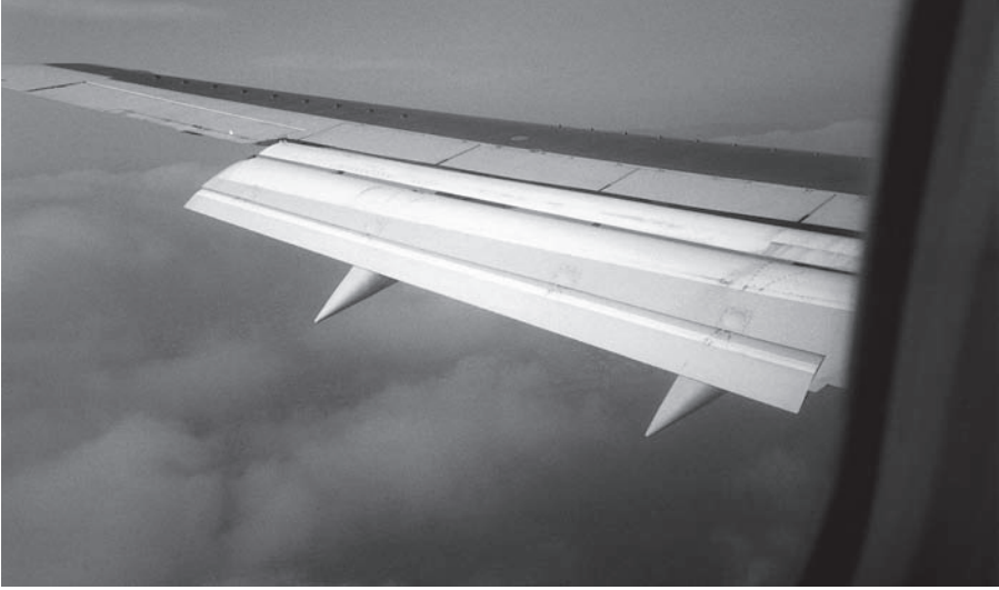
Fig 3H Multi-element slotted flaps Three-element slotted Fowler-type flaps extend rearwards and down as this Boeing 737 prepares to land.
