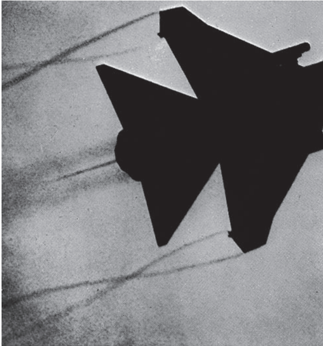
Fig 3B Rolling up of vortices (By courtesy of the former British Aircraft Corporation, Preston) A unique demonstration of the rolling up process; the wing tip and flap tip are each shedding vortices that are strong enough to cause condensation, and the pair roll around one another.
