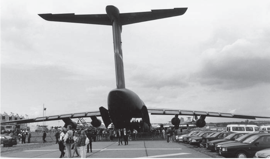
Fig 5F High tail The tail of a Lockheed C-5 Galaxy. The elevators are split into a number of sections to provide redundancy for reasons of safety.
