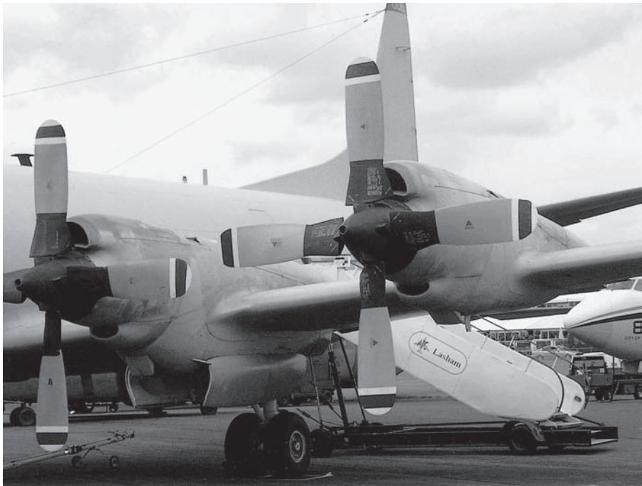
Fig 4B Turboprop propulsion The Lockheed Orion with four turboprops. Note the huge wide-chord 'paddle-blade' propellers.
