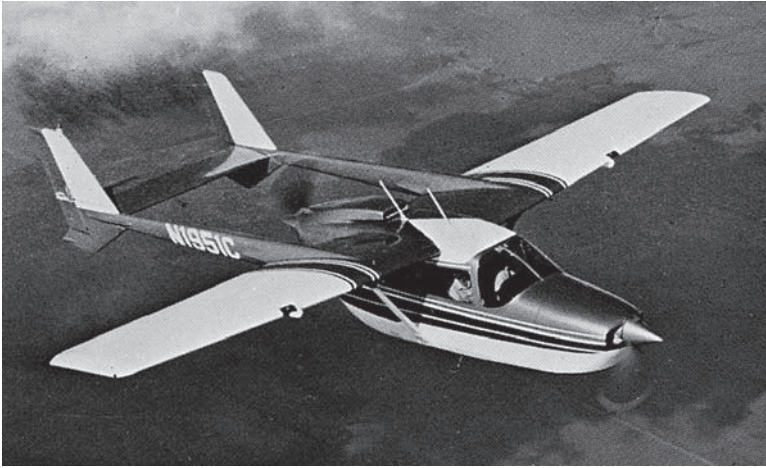
Fig 4H Pusher and tractor (By courtesy of Cessna Aircraft Company, USA) Unique 4/6 seater with two tandem horizontally opposed air-cooled engines, each driving a 2-blade feathering constant-speed propeller.
