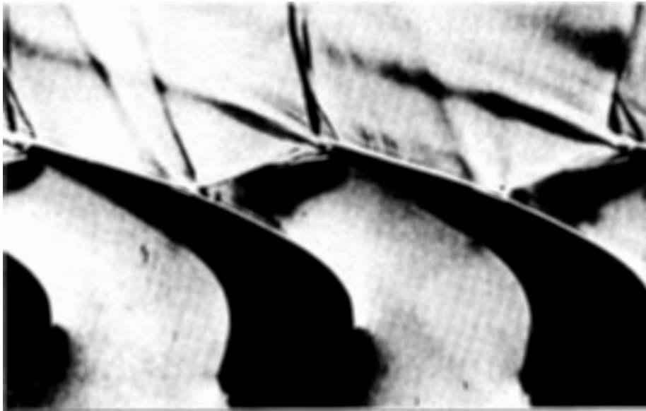
FIGURE 8.11 Schlieren visualization of flow through a linear cascade of high-pressure transonic turbine rotor blades ( 130^\circ turning). A three-color filter was aligned with the suction surface to show details of the shock-laminar boundary layer interaction. The characteristic “tramline” shocks separated by an expansion are clearly visible. Transition occurs on reattachment of the separation bubble. The isentropic outlet Mach number is 1.15, and the Reynolds number is 7 \times 10^5 (based on chord). (Photo by J. J. Camus, Whittle Laboratory, Cambridge, from a research program sponsored by Rolls-Royce.)
