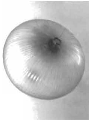
Fig. 8.10. A model isotenoid reinforced along the meridians.
