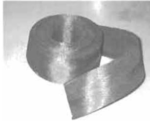
Fig. 4.77. A carbon fabric tape.
