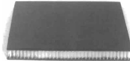
Fig. 5.15. Composite sandwich panel with honeycomb core.
