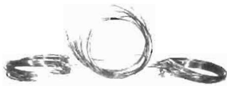
Fig. 3.48. Failure modes of unidirectional rings.
