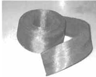
Fig. 4.77. A carbon fabric tape.
