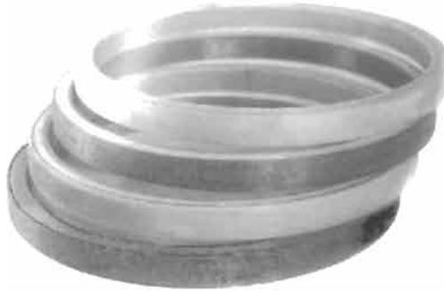
Fig. 5.16. Composite sandwich rings with foam core.
