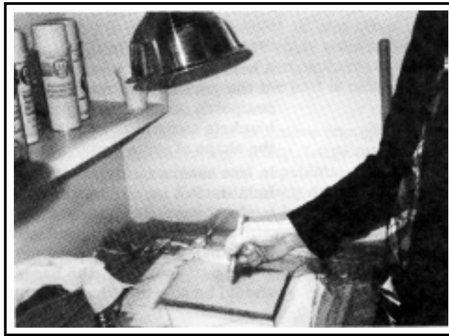
Fig. 11.5, Heat lamps are NOT recommended. They tend to overheat and heat only localized spots.
