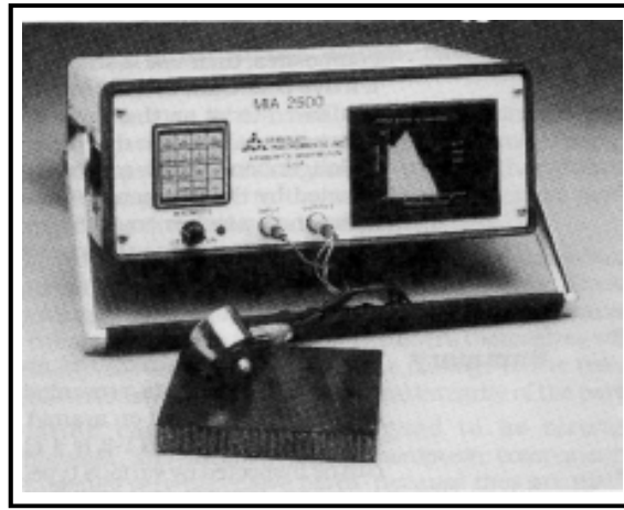
Fig. 12.3, Ultrasonic tester for composite use. (Staveland Instruments).
