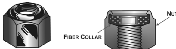
Fig. 18.4, Low-temperature (250°F or less) self-locking nut (elastic stop nut, AN 365, MS20365)
