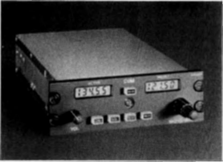
Plate 11 The Becker AR3202 VHF Transceiver for aircraft. This equipment operates on any of 760 channels between 115.0 and 136.975 MHz, one of which may be preselected. The transmitter has an output of 20 W. ( Photo: Becker Flugfunk )
