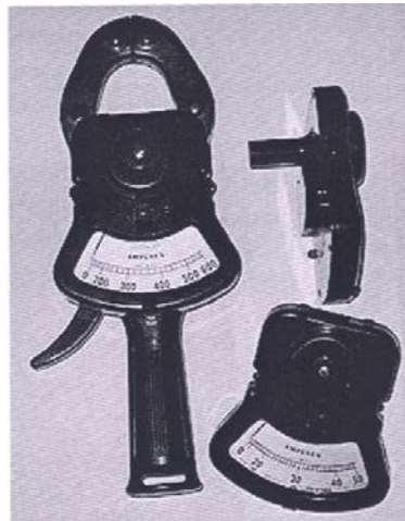
Fig. 10.12, An iron vane type clamp-on ammeter
