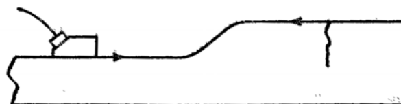
Fig. 32.7, Surface Wave Testing
