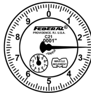
Fig. 3.21, Continuous dial with revolution counter and double dial.
