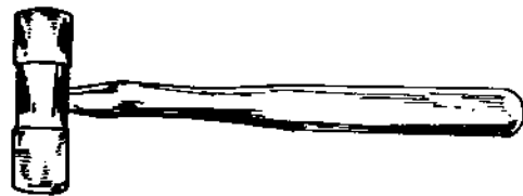
Fig. 2.22 (b), Plastic faced soft hammer.
