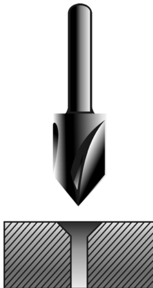
Fig. 4.26, Countersink and countersunk hole.
