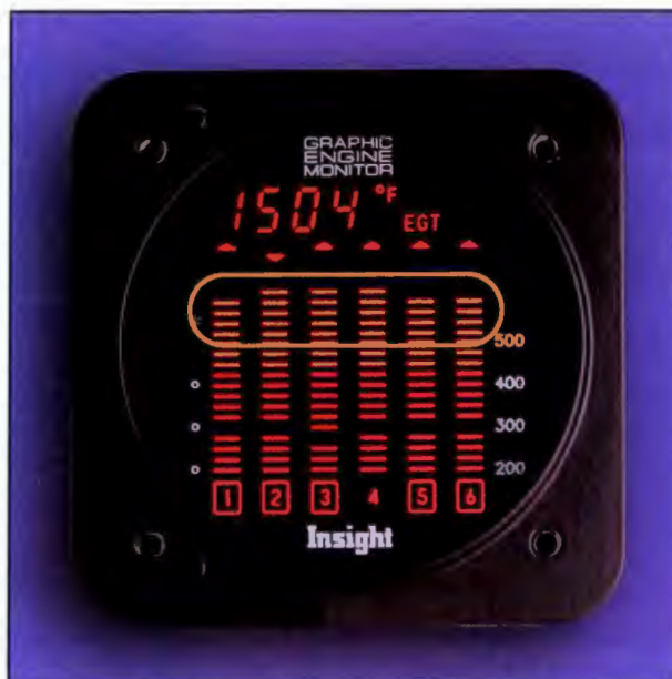
Figure 14-17. An EGT rise in all cylinders may be the result of a failed magneto.
