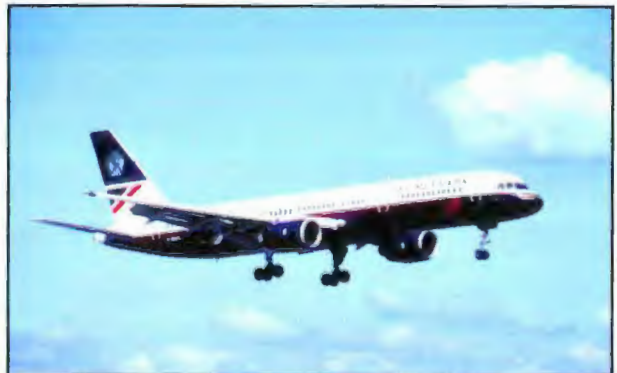
Figure 5-18. A Boeing 757 has wing-mounted engines that use engine-mounted inlet ducts directly in front of the compressor.
