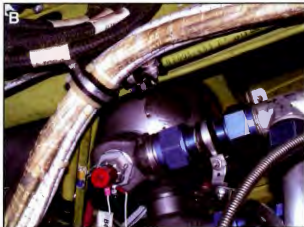
Figure 13-24. (A) Fire detection elements are inspected for condition and security of attachment. (B) Fire suppression systems are checked for weight and state of charge. Also check the expiration date on discharge cartridges or squibs.
