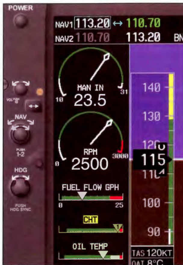
Figure 2-2. Digital flight displays present engine performance information intuitively and efficiently.
