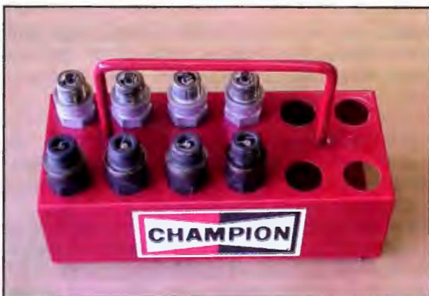
Figure 8-148. Spark plug trays provide a secure, organized place to store spark plugs when you remove them for service.
