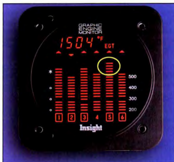
Figure 14-15. A rise in EGT in one cylinder may be the result of a lean mixture in that cylinder.
