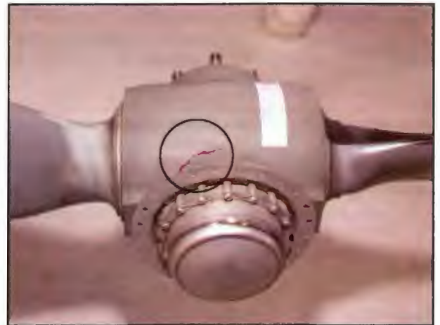
Figure 13-26. For some constant-speed propellers, red-colored oil coming from the propeller hub is indicative of a crack. If red oil is detected, the propeller must be removed for servicing at an authorized propeller repair facility.
