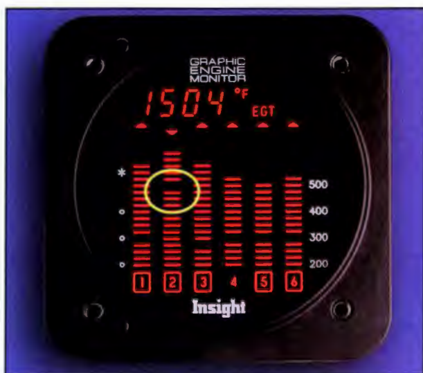
Figure 14-16. A high CHT in one cylinder may be the result of cracked cylinder fins.
