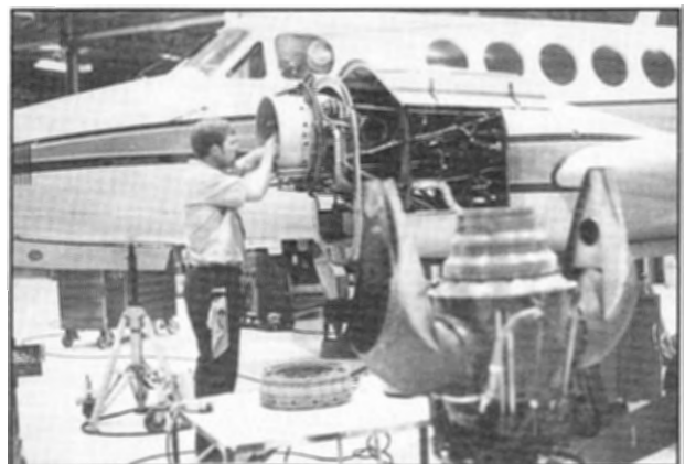
Figure 4-22. The modular design of some turboprop engines makes it possible to perform many maintenance tasks with the engine attached to the aircraft.
