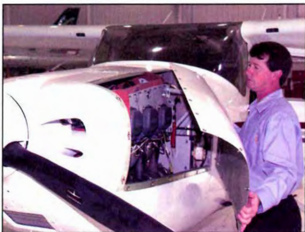
Figure 13-11. With the engine cowling removed, do a quick visual inspection before starting the engine. Write down any discrepancies that you find during the inspection.
