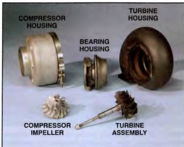
Figure 5-9. A turbocharger consists of a compressor impeller and a turbine mounted on a single rotating shaft. Both the impeller and turbine are surrounded by separate housings joined by a common bearing housing.
