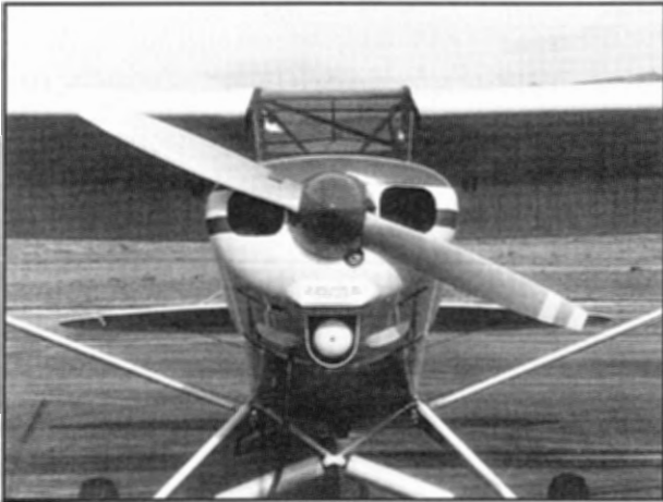
Figure 12-83. When installing a propeller on a four-cylinder opposed engine, one of the blades should come to rest at the ten o'clock position to reduce vibration and facilitate hand propping.
