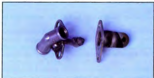
Figure 13-19. One of the most critical items for promoting proper turbine engine operation and optimum service life is to check that the fuel nozzles are clean and in good condition. This is done by periodically removing the nozzles and performing a flow check. Dirty nozzles can produce fuel streaking, which can cause severe damage to hot section components.
