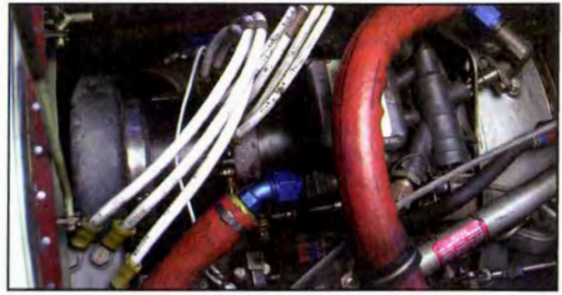
Figure 13-23. Electrical starter/generator wiring and connections must be secure to prevent abrasion, and free of corrosion or other defects.
