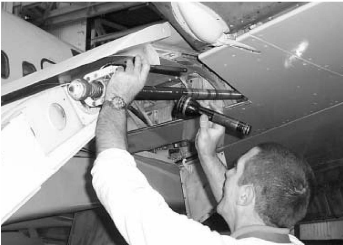
Use of artificial lighting to supplement the ambient illumination in hanger
