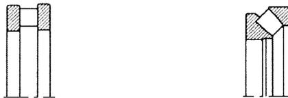
Cylindrical roller thrust bearing    Spherical roller thrust bearing
