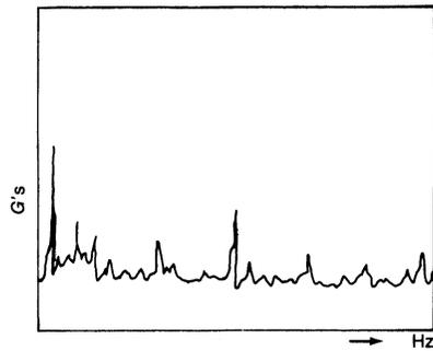
Figure 7-39. Fifth-stage bleed pressure—5800 rpm.
