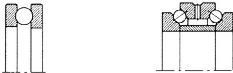
Thrust ball bearing    Angular contact thrust ball bearing double direction
