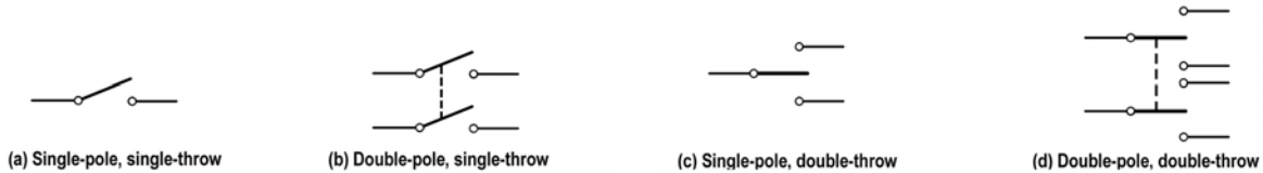
Fig. 7.1. Switch contact arrangements.
