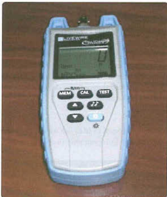
Figure 4-5. An SSTDR showing an open at 0 feet.
