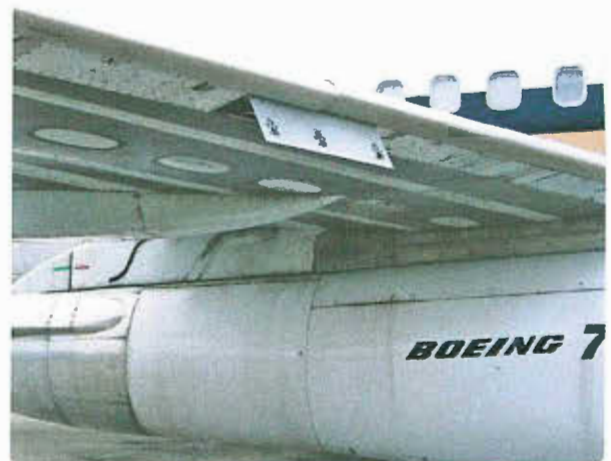
Figure 17-27. Single point refueling station of a large aircraft.
