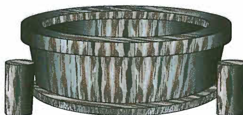
Figure 11-7. Etching and corrosion appears as a reddish/brown discoloration.
