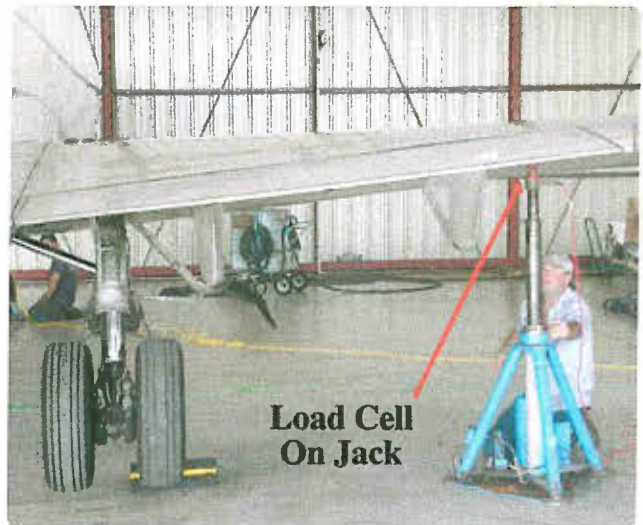
Figure 16-15. Airplane on jacks with load cells in use.
