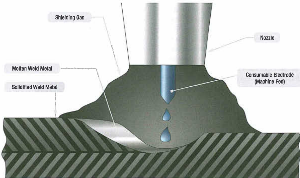
Figure 15-5. Metal inert gas (MIG) welding process.
