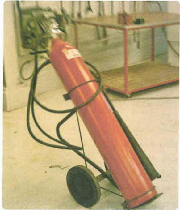
Figure 1-5. Carbon dioxide fire extinguisher.
