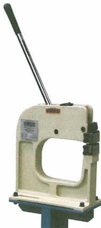
Figure 3-90. Hand operated shrinker and stretcher unit.
