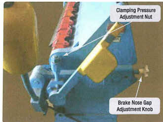
Figure 14-24. Adjust clamping pressure with the clamping pressure nut radius shims.
