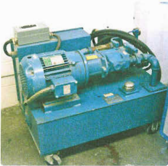
Figure 17-23. A portable hydraulic power unit.
