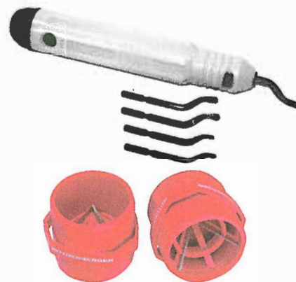
Figure 9-2. Deburring tool types.
