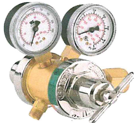
Figure 15-15. Two-stage oxygen regulator. No groove on the cylinder connection nut indicates a right hand thread.
