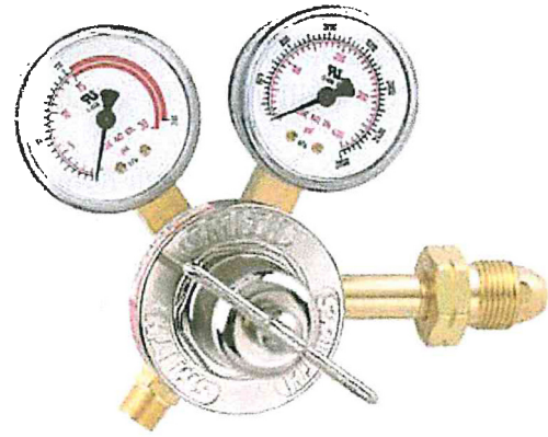
Figure 15-14. Single-stage acetylene regulator. Note the maximum 15-psi working pressure. The notched groove cylinder connection nut indicates a left hand thread.
