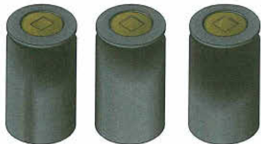
Figure 11-3. Overheating results in a bluish tint to the metal surface.
