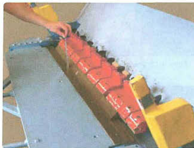
Figure 14-25. Brake nose gap adjustment with piece of material same thickness as part to be formed.
