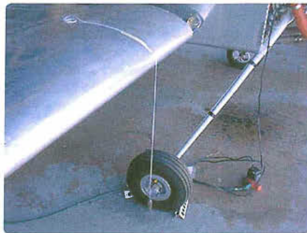
Figure 16-17. Plumb bob dropped from a wing leading edge.
