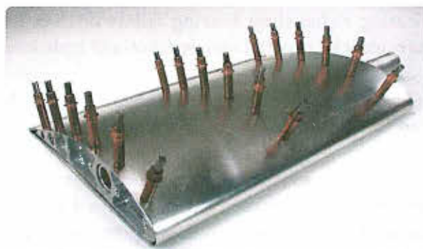
Figure 8-26. A part temporarily held together with Cleco fasteners.
