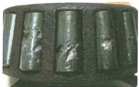
Figure 11-2. Spalling is a chipped away portion of the hardened surface.
