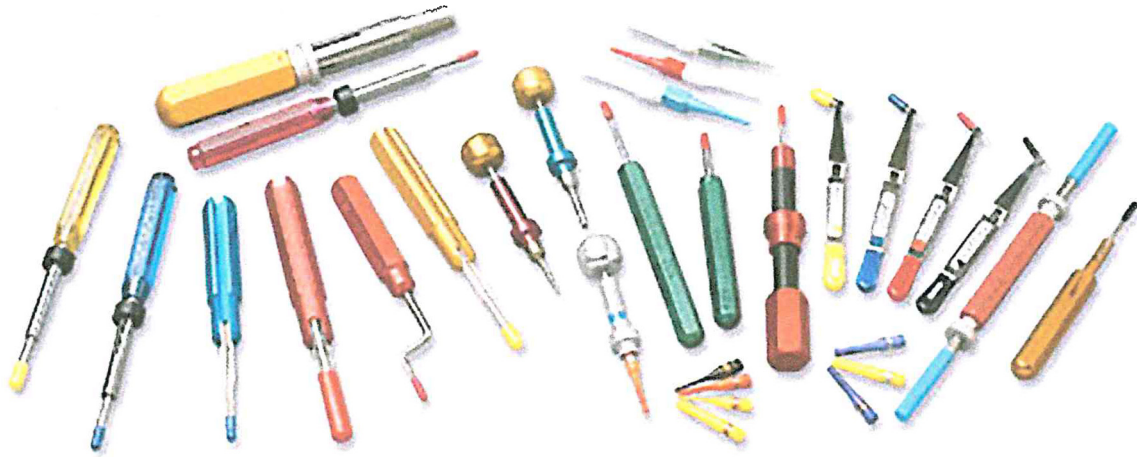
Figure 7-17. Typical pins and associated insertion tools.
