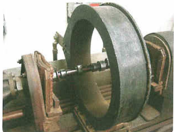
Figure 18-52. Longitudinal magnetization of camshaft (solenoid method).
