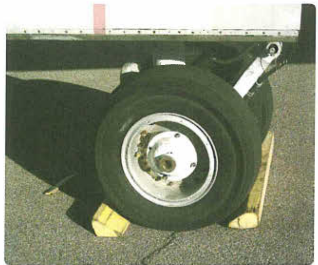
Figure 17-4. Wheels chocked fore and aft.
