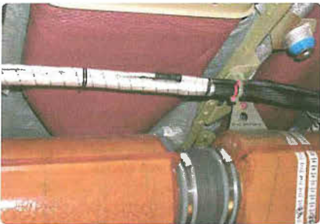
Figure 7-45. Shielded wire harness for flight control.
