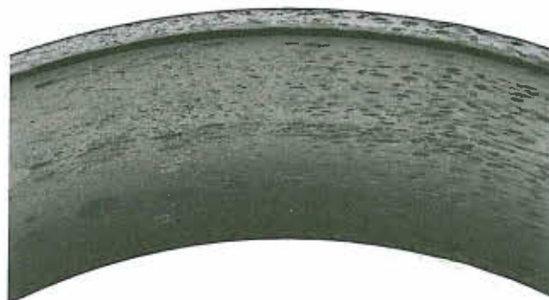
Figure 11-8. Bruising leaves a less than smooth surface on the bearing cup.
