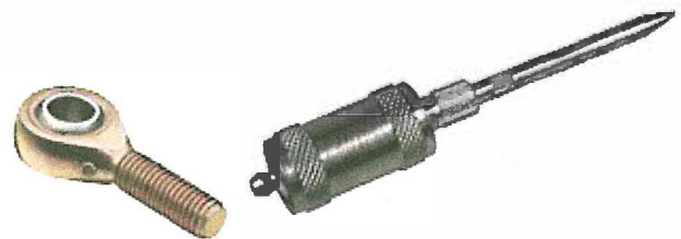
Figure 3-95. Flush mount grease fitting for a rod end bearing and grease gun tip.
