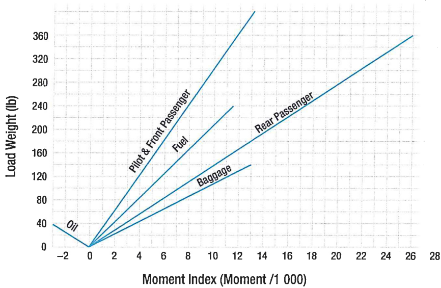
Figure 16-30. Aircraft loading graph.
