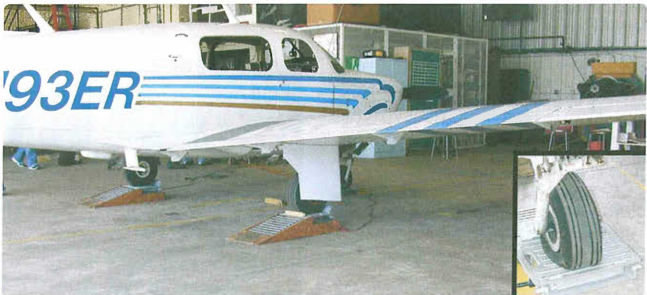
Figure 16-13. Mooney M20 being weighed with portable electronic platform scales.
