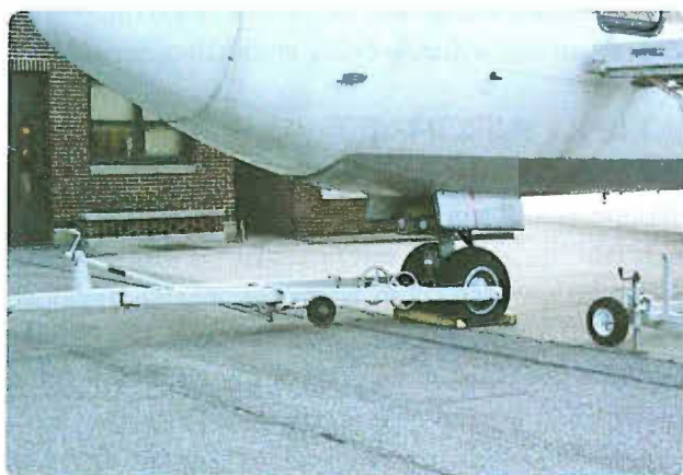
Figure 17-14. Tow bar for a large aircraft.
