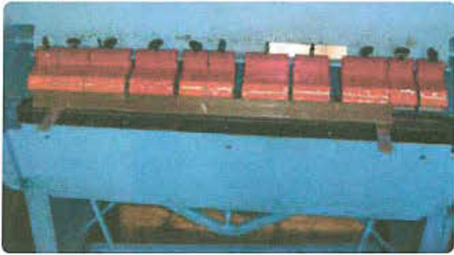
Figure 14-27. Brake alignment with two test strips 3-inches from each end.
