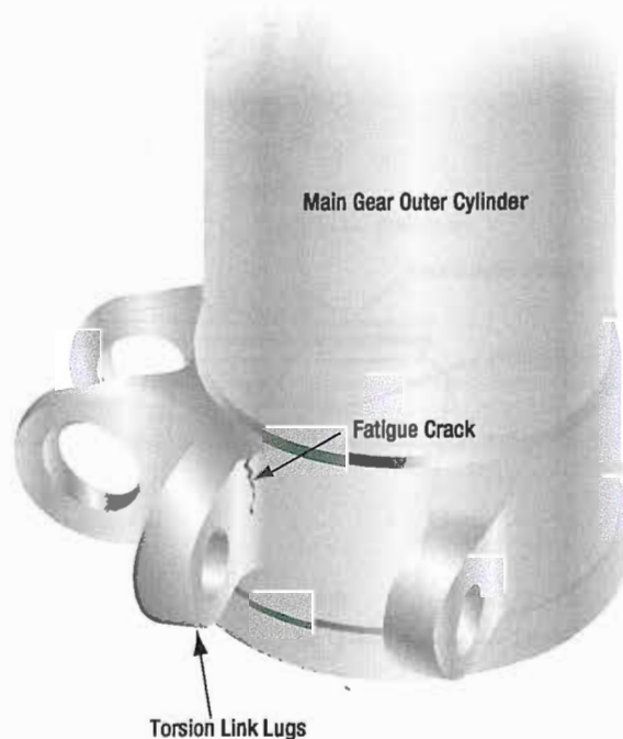
Figure 18-53. Fatigue crack in a landing gear.
