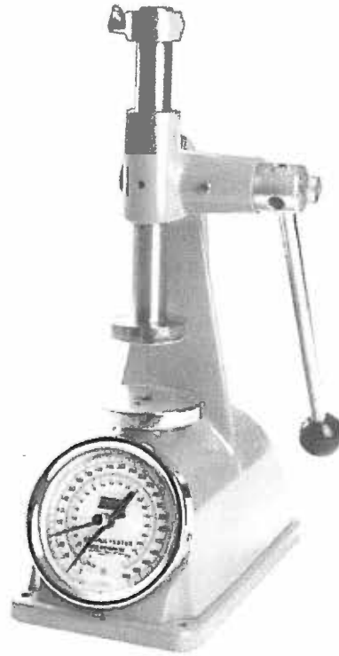
Figure 10-1. A spring compression tester.
