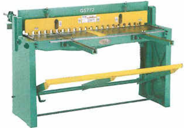
Figure 3-50. Foot-operated squaring shear.
