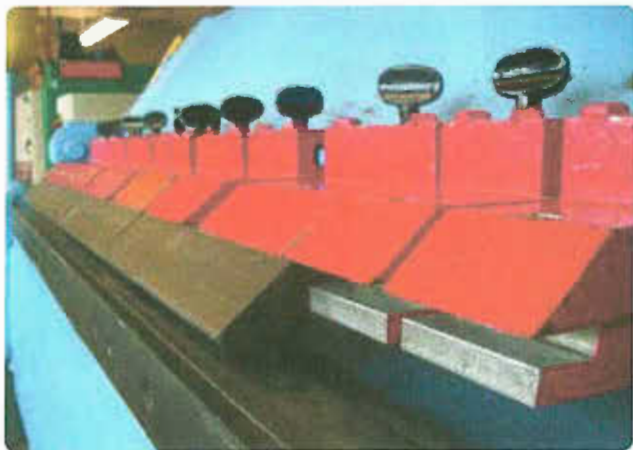
Figure 14-20. Brake radius nose piece adjustment.
