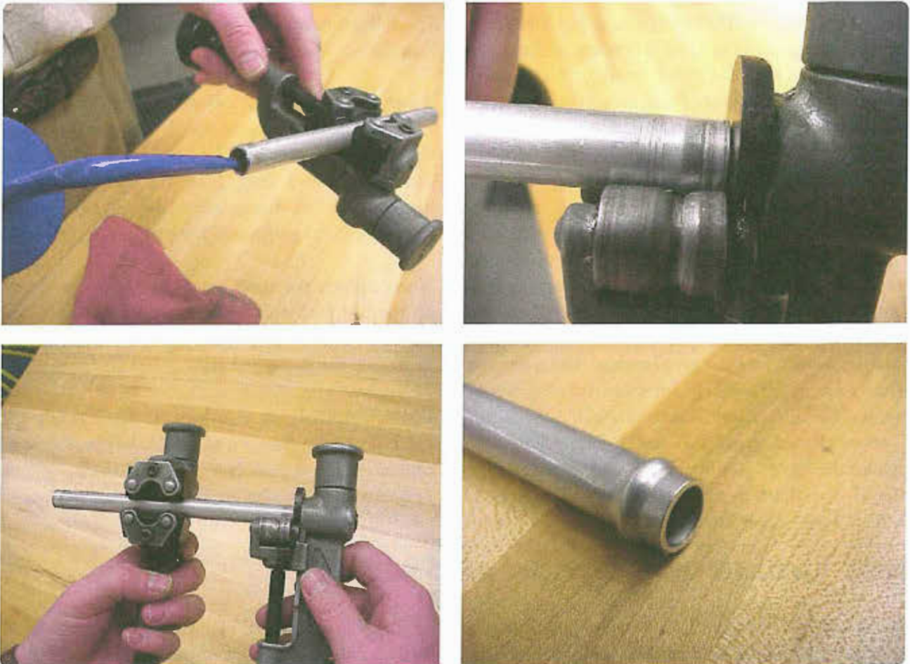
Figure 9-11. Hand beading tool.
