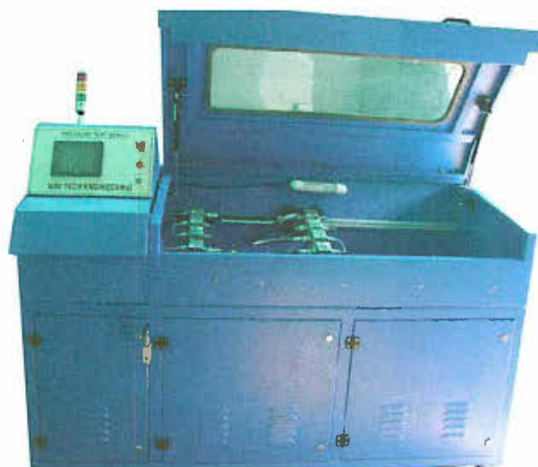
Figure 9-19. Hydraulic hose burst test stand.
