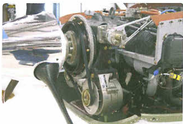
Figure 12-4. An alternator drive belt on a piston aircraft engine.
