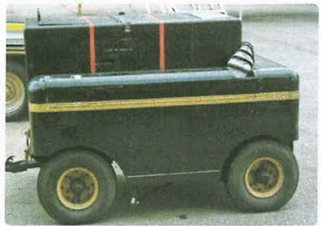
Figure 17-24. A portable compressed air cart.
