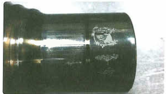
Figure 11-1. Galling is caused by rubbing of mating surfaces.
