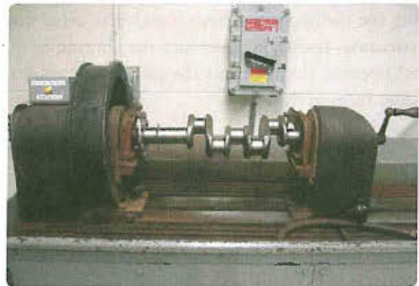
Figure 18-51. Circular magnetization of a crankshaft.
