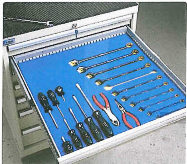
Figure 2-1. Foam draw liner where every tool has its place.
