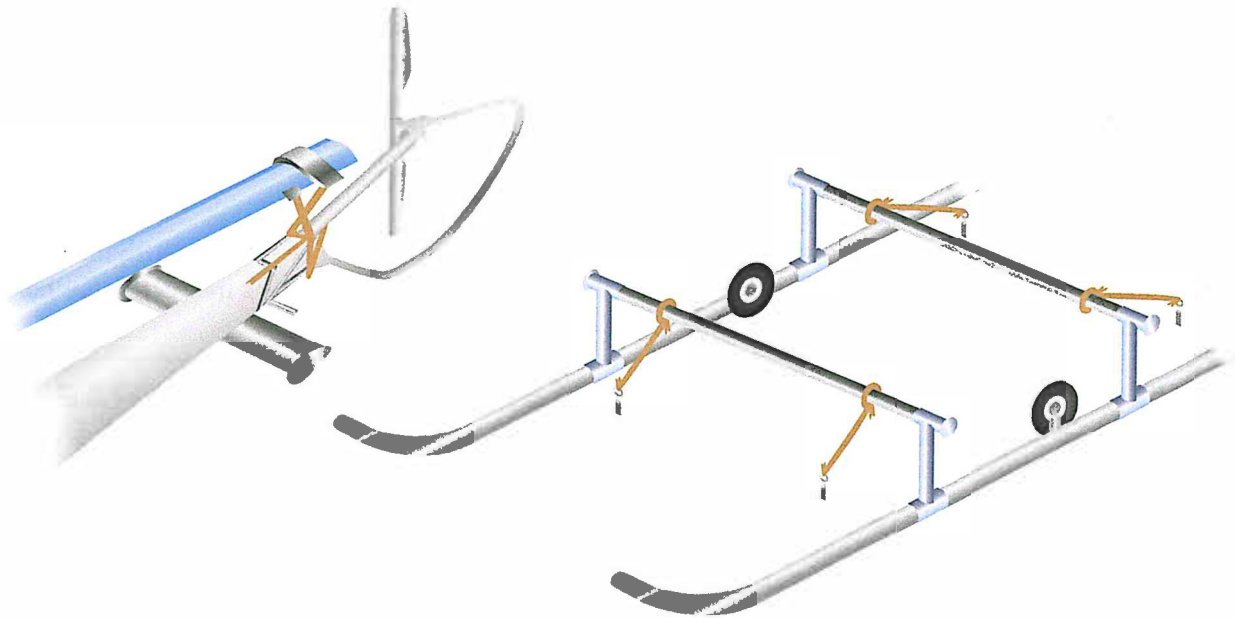
Figure 17-6. Securing helicopter blades and fuselage.
