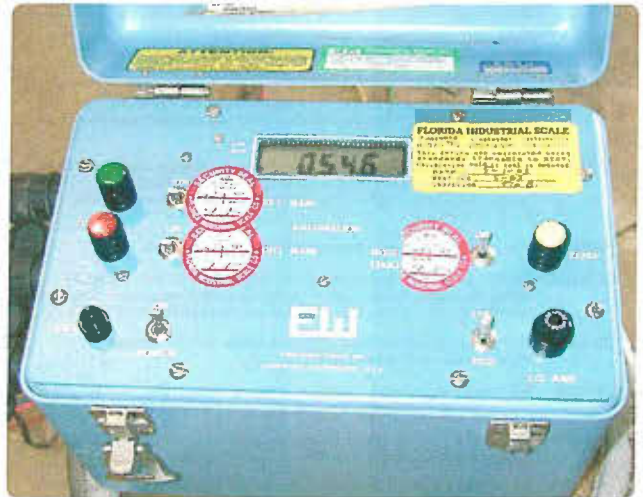
Figure 16-14. Display unit showing nosewheel weight for Mooney M20.
