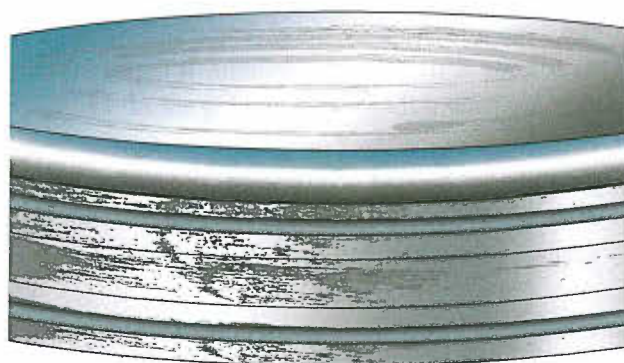
Figure 11-9. Bearing cups spinning in the wheel is shown.
