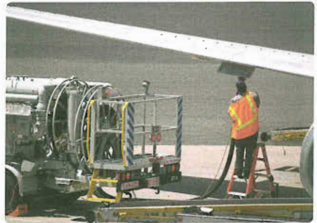
Figure 17-26. Refueling an aircraft by the over-the-wing method.
