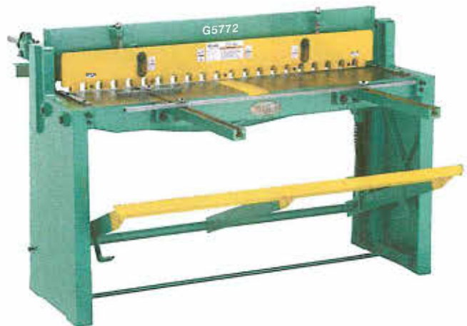
Figure 3-50. Foot-operated squaring shear.
