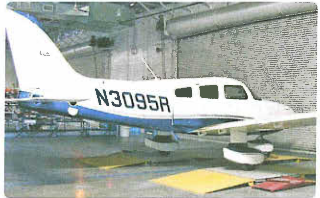
Figure 16-12. Weighing a Piper Archer using electronic platform scales.
