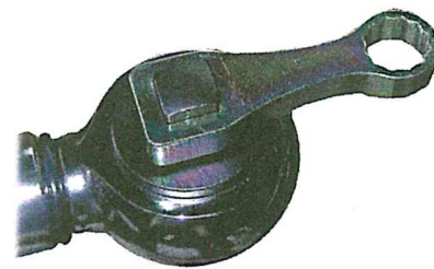
Figure 3-27. A typical torque wrench extension in the straight position.
