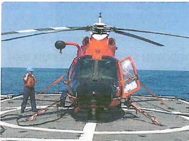
Figure 17-5. Example of mooring of a helicopter.
