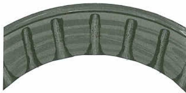
Figure 11-6. Staining and surface marks on the bearing.
