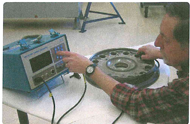
Figure 18-40. Eddy current inspection of wheel half.
