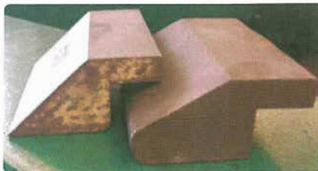
Figure 14-21. Interchangeable brake radius bars.
