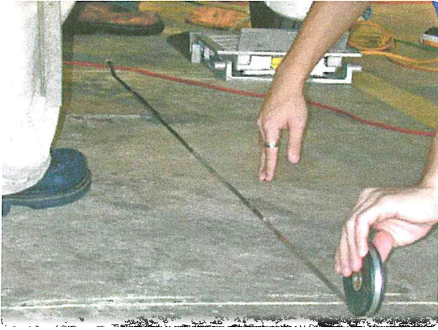
Figure 16-18. Measuring the nosewheel arm on a Cessna 310.
