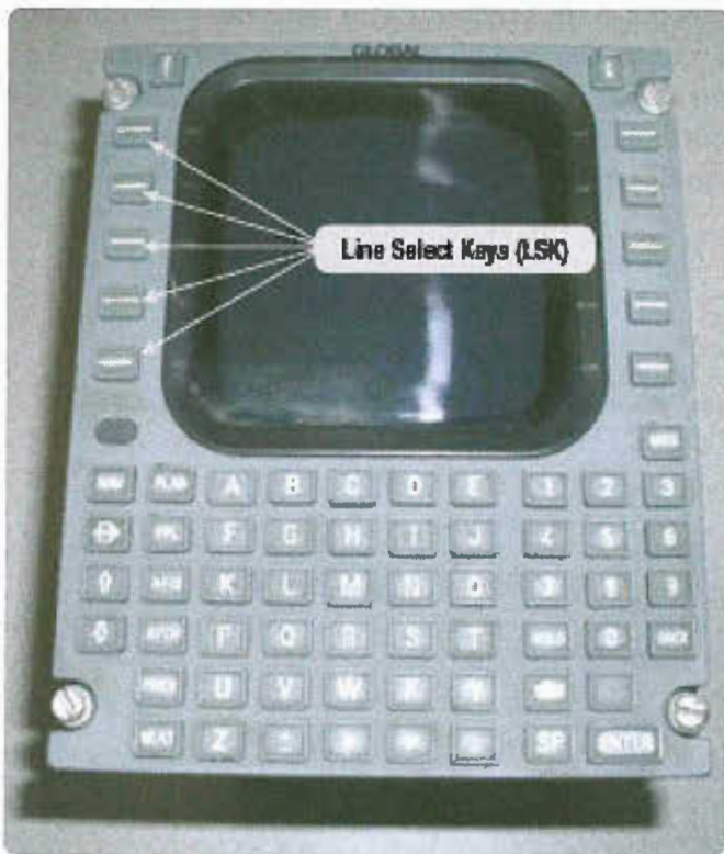
Figure 4-2. Line select keys (LSK) used for selecting options while interrogating the central maintenance computer on the CDU.
