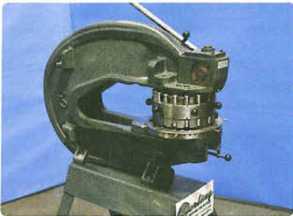
Figure 3-49. Rotary punch press.
