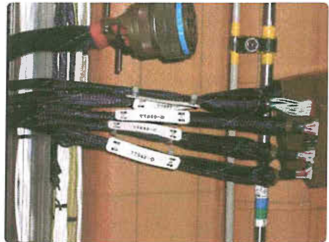
Figure 7-29. Alternate method of identifying wire bundles.
