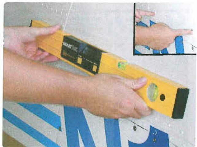
Figure 16-16. Spirit level being used on a Mooney M20.
