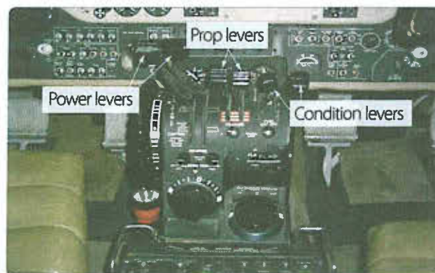
Figure 17-10. Engine controls of a turboprop aircraft.
