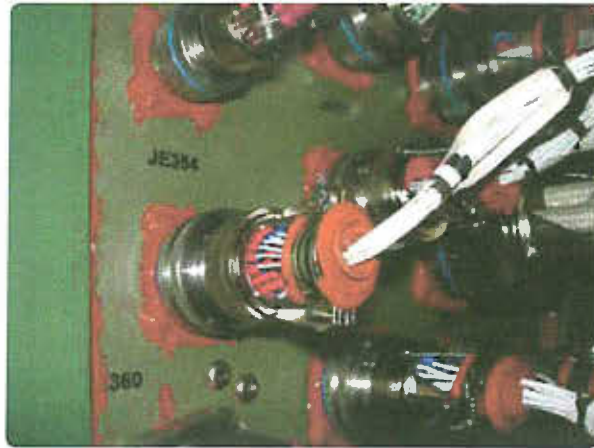
Figure 7-22. Backshells with strain relief.
