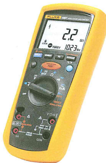
Figure 7-1. An insulation tester.
