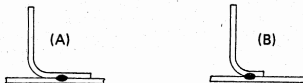
Figure 2 ATTACHMENT OF STRINGERS TO SHEETS
