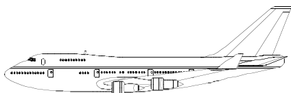
B747-400 long-haul airliner 4 \times 58\,000 lbf (258.6 kN) turbofan
