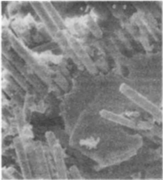
Figure 9-32. Photograph of fibers pulled out of matrix in a glass-epoxy composite (600X).
