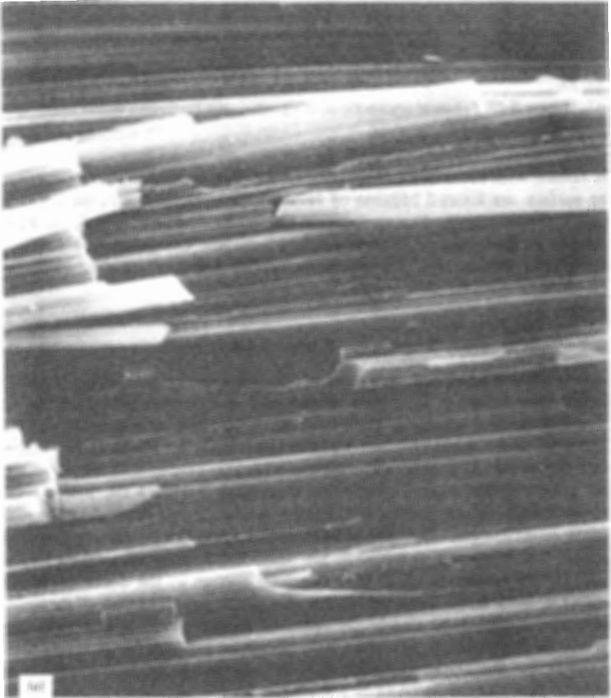
Figure 3-28. Photomicrographs of fracture surfaces of unidirectional graphite-fiber composites failed under transverse tensile loads with fibers being (a) high modulus and (b) high tensile strength. (From Chamis et al. [46].)
