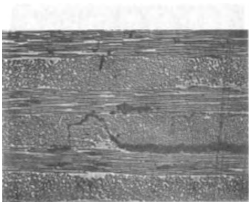
Figure 9-3. Longitudinal-ply crack appears in a cross section.
