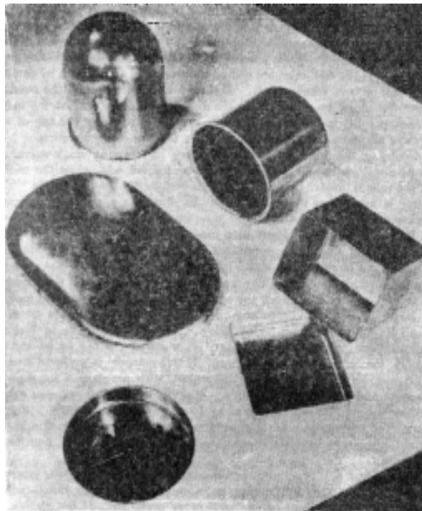
Fig.8.9. Drawn Magnesium Parts
