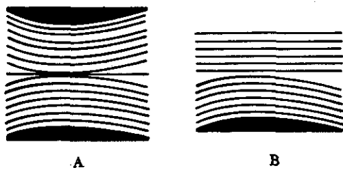
FIGURE 7-22. Airflow in venturi sections.
