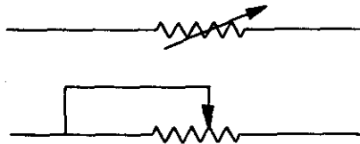
FIGURE 8-36. Symbols for variable resistors.
