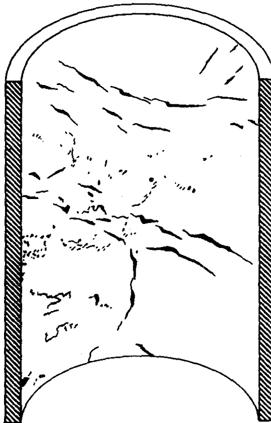
FIGURE 10-9. Heat-treat cracks on cylinder barrel wall.
