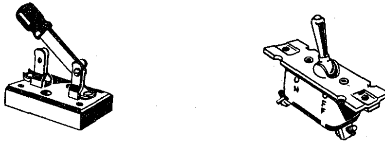
FIGURE 8-112. Single-pole single-throw knife and toggle switches.
