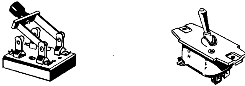
FIGURE 8-114. Double-pole single-throw knife and toggle switches.
