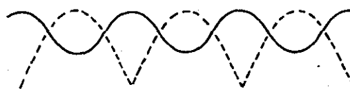
FIGURE 8-248. Output of an inductor filter rectifier.
