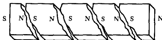
FIGURE 8-89. Magnetic poles in a broken magnet.
