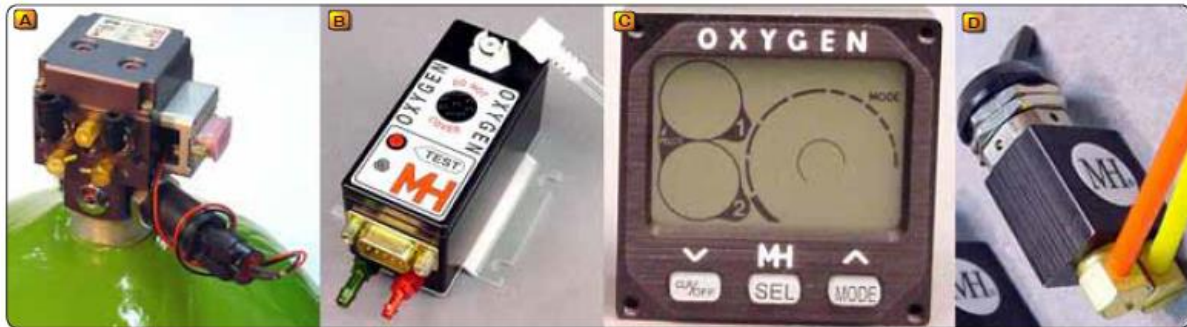
The key components of a built-in electronic pulse demand oxygen metering system: (A) electronic regulator, (B) oxygen station distributor unit, (C) command/display unit, (D) emergency bypass switch.
