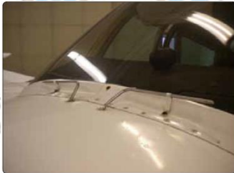
Chemical deicing spray tubes.
