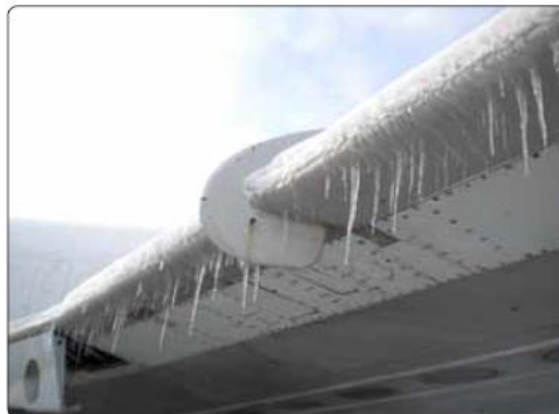
Formation of ice on aircraft leading edge.
