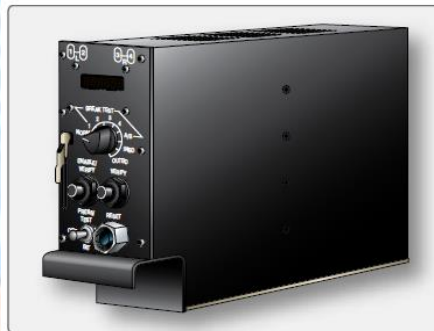
A rack mounted antiskid control unit from an airliner.
