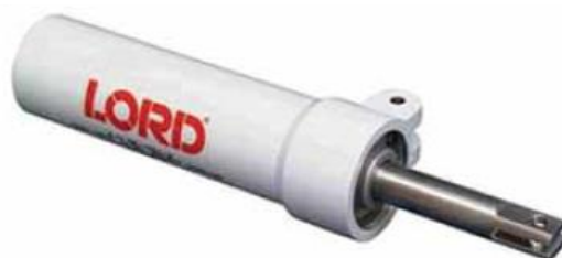
A non-hydraulic shimmy damper uses a rubber piston with lubricant that dampens via motion against the inner diameter of the unit housing.
