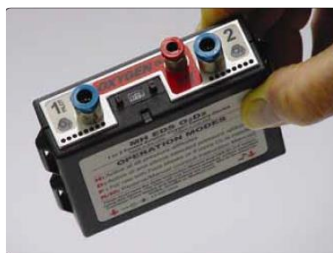
A portable two-person electronic pulse-demand (EPD) oxygen regulating unit.
