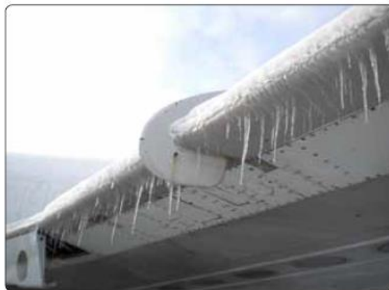
Formation of ice on aircraft leading edge.
