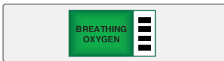
Colour-coded tape used to identify oxygen tubing.
