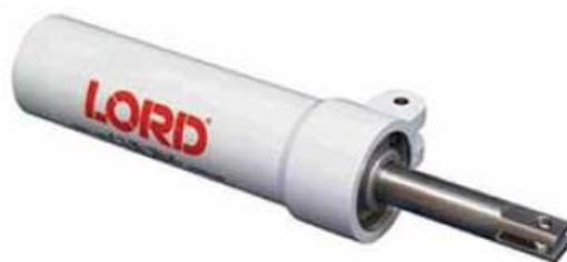
A non-hydraulic shimmy damper uses a rubber piston with lubricant that dampens via motion against the inner diameter of the unit housing.
