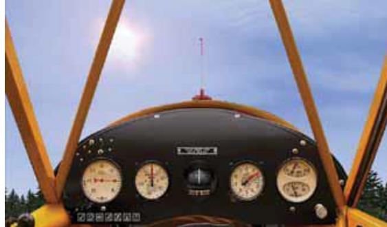
The fuel quantity indicator on this Piper Cub is a float attached to a rod that protrudes through the fuel cap.
