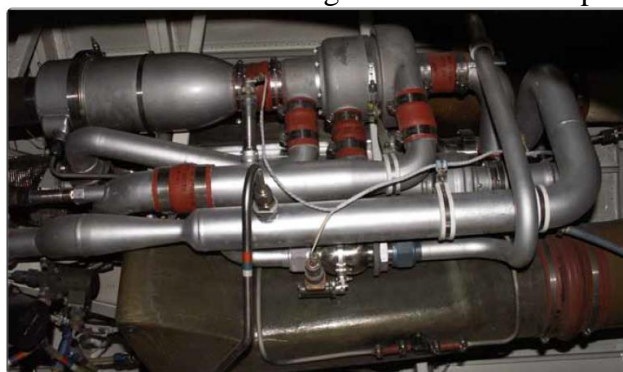
An air cycle air conditioning system used to pressurize the cabin of a business jet
