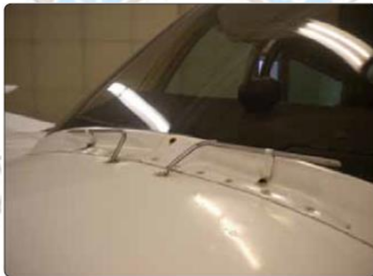
Chemical deicing spray tubes.
